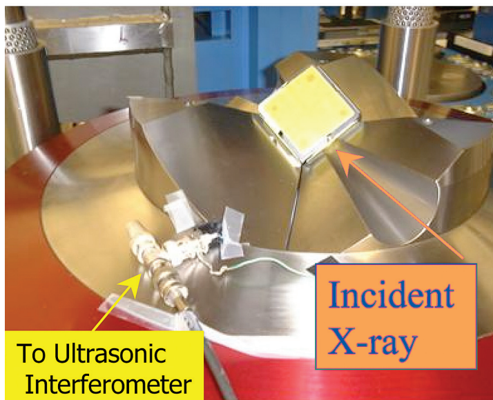
FIGURE 5 A Kawai-type multi-anvil apparatus at the Advanced Photon Source, ready for an ultrasonics experiment in which the elastic properties and density will be measured at high pressures and temperatures. In the bottom picture, the X-rays coming from the right are incident on a sample embedded in the center of 8 tungsten-carbide cubes (hidden in this photograph). See Bass et al. (2008 this issue) for additional details. AFTER LI ET AL. (2005)
