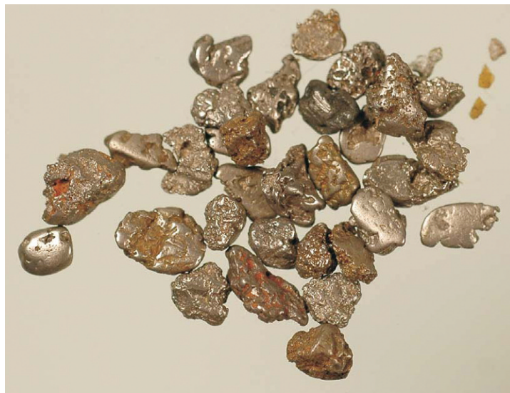
FIGURE 3 Samples of "platina" recovered from the placer deposits in the Choco district of Colombia. Similar material was described by William Lewis to the Royal Society of London in 1754 and served as the feedstock for the first purification of Pt, Pd, Ir, and Os by Smithson Tennant and William Wollaston. The field of view is 5 cm wide (each nugget is about 3–5 mm in length). Sample is from the mineralogy collection of the Museum National d'Histoire Naturelle (#4.283; Picture D. Brabant, MNHN). PHOTO COURTESY OF JEAN-PIERRE LORAND
