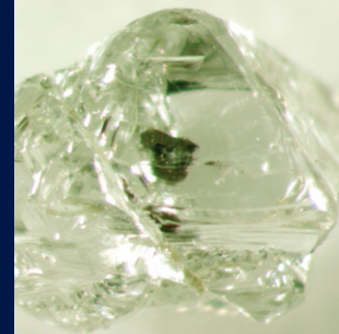
Photomicrograph of diamond with Fe-sulfide inclusion
