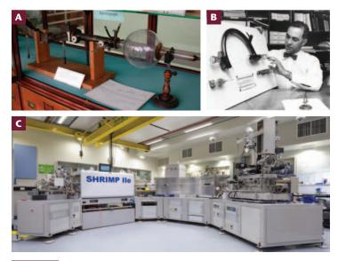
(A) Aston's third mass spectrograph, used for Pb FIGURE 2 isotope analysis (COURTESY OF CAMBRIDGE PHYSICS OUTREACH); (B) Alfred Nier with the flight tube of his 180° mass spectrometer, used to measure the isotopic composition of uranium (UNIVERSITY OF MINNESOTA, COURTESY OF AIP EMILIO SEGRE VISUAL ARCHIVES); (C) for comparison, a modern SHRIMP IIe SIMS instrument (SOURCE: GEOSCIENCE AUSTRALIA)
