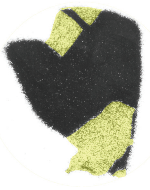
Figure 2.4 Fission track map of Pu partitioning between diopside and liquid (modified from Jones, 1981). Blackest areas signify the highest Pu concentrations ( i.e. glass). Three pyroxene crystals can be observed. The spatial scale of the largest pyroxene crystal is a few hundred microns. The ^{Pu}D_{pyx/liq} is about 0.17.
