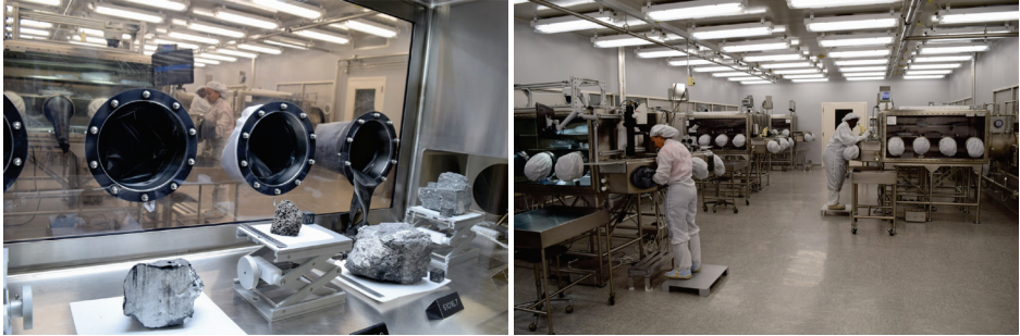
Figure 7. (left) A view of four large Apollo samples on display in the Pristine Apollo Sample Processing Laboratory at Johnson Space Center (left to right samples are 60015,1; 15016,0; 61016,7; and 15459,0). All pristine lunar samples are processed in stainless steel glove boxes using only stainless steel, aluminum, or Teflon tools in an ultra-pure dry N_2 gas environment. (right) A view of Apollo sample processors Andrea Mosie (right) and Charis Krysher (left) working in the Pristine Apollo Sample Processing Laboratory at NASA Johnson Space Center.
