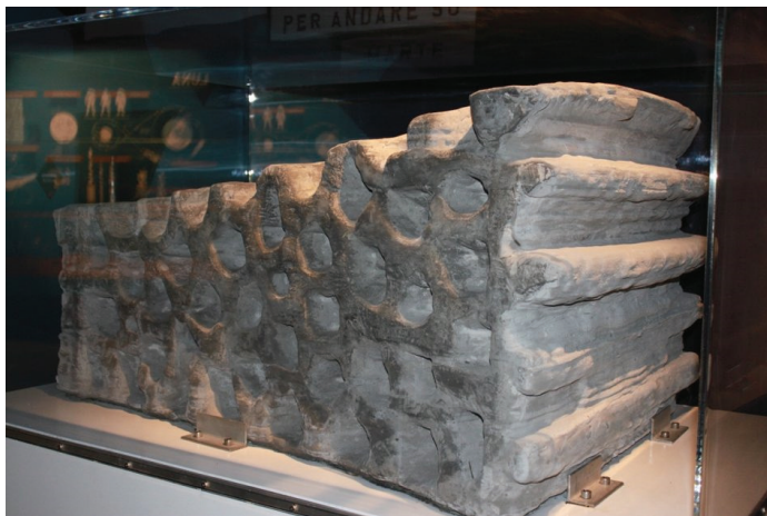
Figure 5. A ~1.3 tonne building block produced as a demonstration of 3D printing techniques using lunar regolith simulant (Cesaretti et al. 2014); the overall length of the block is approximately 1.4 m. Image courtesy of ESA.
