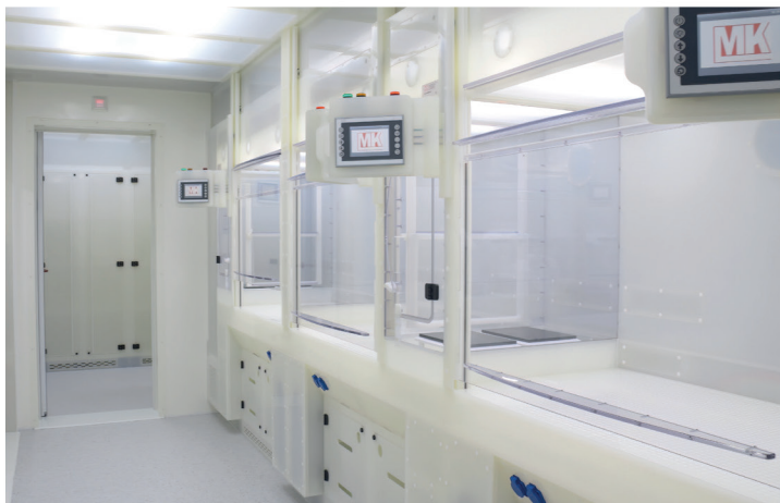
Special laminar flow fume hoods for acid distillation and sample preparation.
