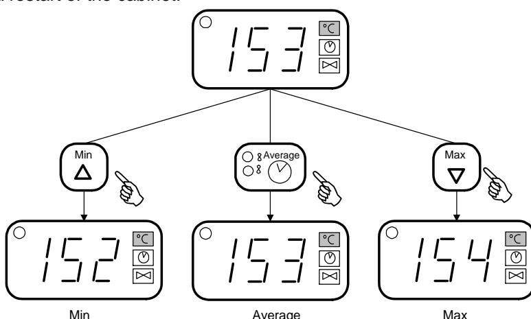
The calculations are done on a minute basis, and starts about 32 minutes after the initial temperature stabilising. In this initial period, " - - " will be displayed if any of those buttons are pressed. Therefore, the datalogging will never start at cycles less than 32 minutes.
