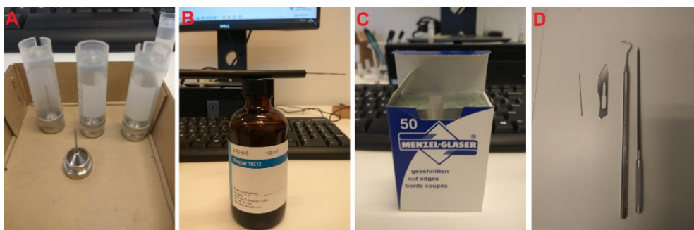
Fig. 23. View of the cryoloop (A), oil (B), glass slides (C) and tools (D) used to mount the samples.
