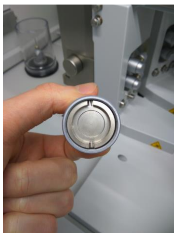
Fig. 6. View of the back of the goniometer head.
