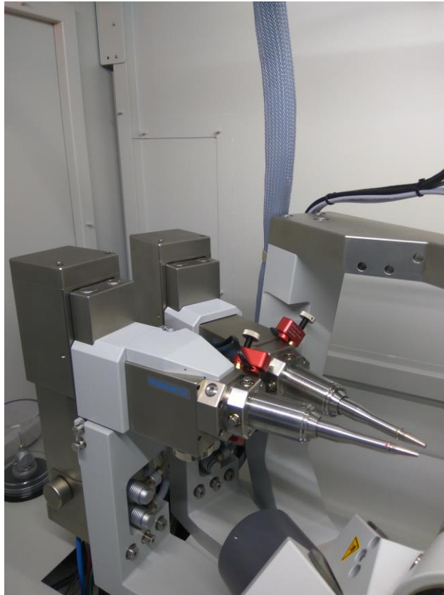
Fig. 2. Detailed view of the Cu (first plan) and Mo (second plan) PhotonJet-S microfocus sealed tube X-ray sources.
