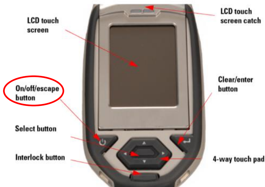
Figure 4: The control panel.
