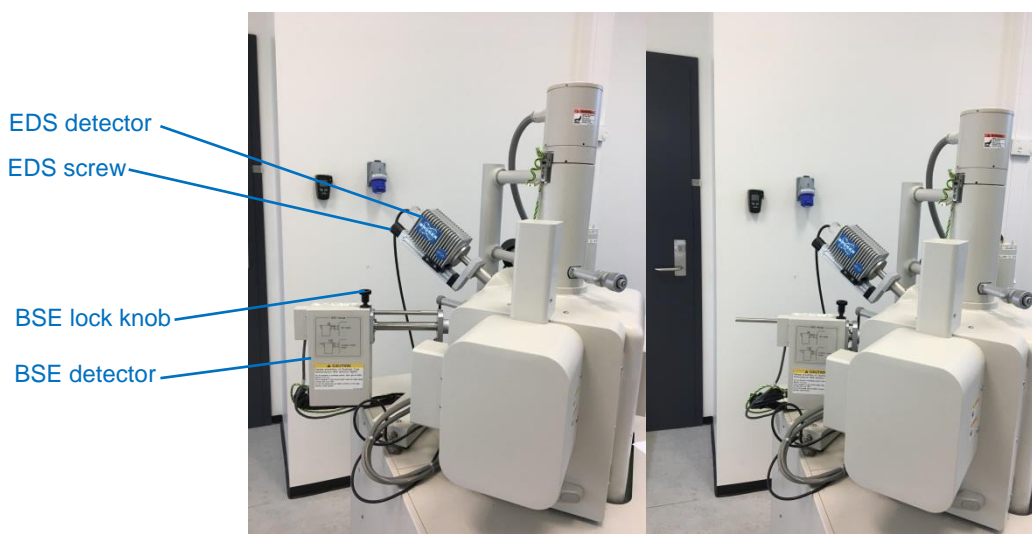
Fig. 5: Detail of the column where BSE and EDS detectors are visible. BSE detector can be seen in the position OUT (left) and COMPO/TOPO (right). EDS detector it is in INN position in both images.
