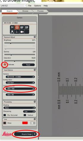
Configuring: When using the software for the first time you might have to configure some settings. These settings will then be remembered. Use JPG, highest quality, for your images. Remember to configure the system (camera, magnification, objectives etc.). Scale bar must be re-calibrated after a possible re-install. If reinstall is required, then select this microscope: DM2500P (most similar to the old DMLP). Remember then to configure scale bars.
